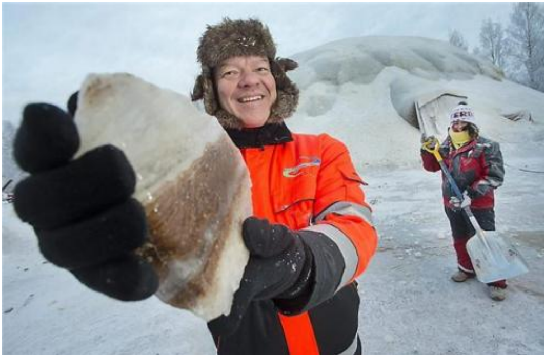
Project leader Arno Pronk shows a piece of pykrete; ice reinforced with wood fibers. Credit: Bart van Overbeeke.
