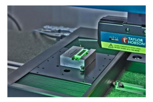
The King of Shaves razor blade cartridge in the dedicated mounting fixture being measured with the Taylor Hobson Form Talysurf PGI instrument
