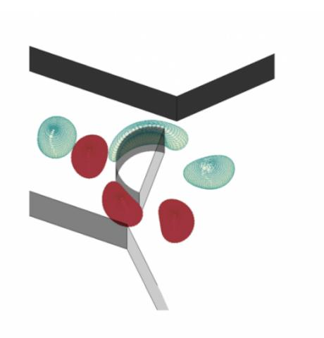
Visualization from a numerical simulation of a cell flowing past the obstacle through the microfluidic device.
