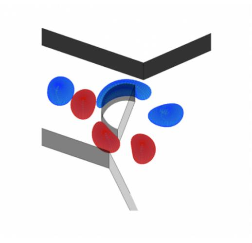
Visualization from a numerical simulation of a cell flowing past the obstacle through the microfluidic device.
