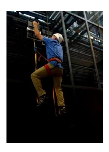
During testing, an operator climbed 25 feet vertically on a glass surface using no climbing equipment other than a pair of hand-held, gecko-inspired paddles. The climber wore, but did not require, the use of a safety belay. Credit: DARPA
