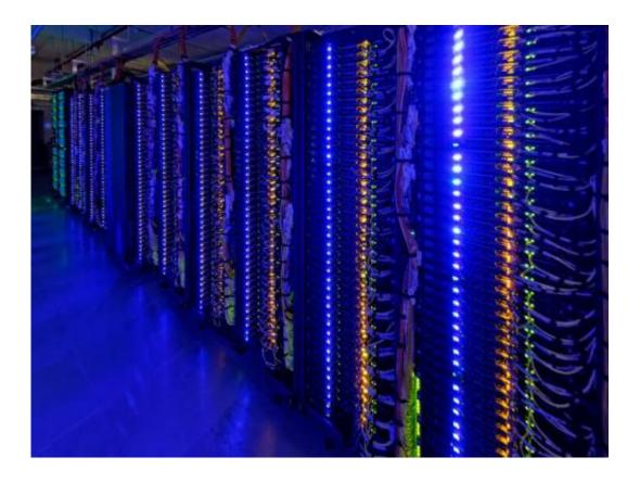
Description: The DiRAC Cosmology Machine, operated by Durham University has 6720 Intel Xeon Cores and 53,760 GByte of RAM. Credit: Till Sawala, Durham University
