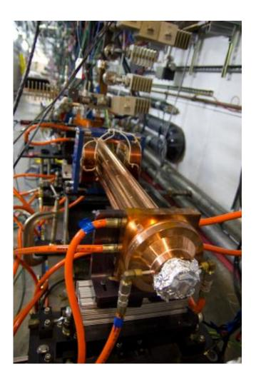
This microwave undulator, designed and built at SLAC, uses microwave power and electrons to produce shorter-wavelength pulses, and is highly tunable compared to conventional undulators that use magnets. Credit: Glenn Roberts Jr./SLAC
