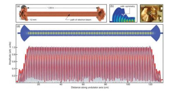
Top: This diagram shows a cutaway view of a microwave undulator designed and built at SLAC, with the path of the electron beam shown in white. (Bottom) Measurement of the electrical field traveling through the magnetic undulator (red), and a simulated view of the electromagnetic field created inside the undulator (blue) by the microwaves propagating through it. Credit: Physical Review Letters/10.1103/PhysRevLett.112.164802
