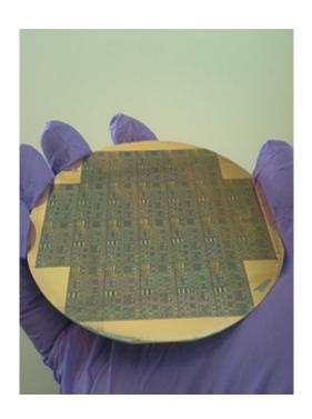
The silicon-carbide wafer contains more 1000 individual circuits.
