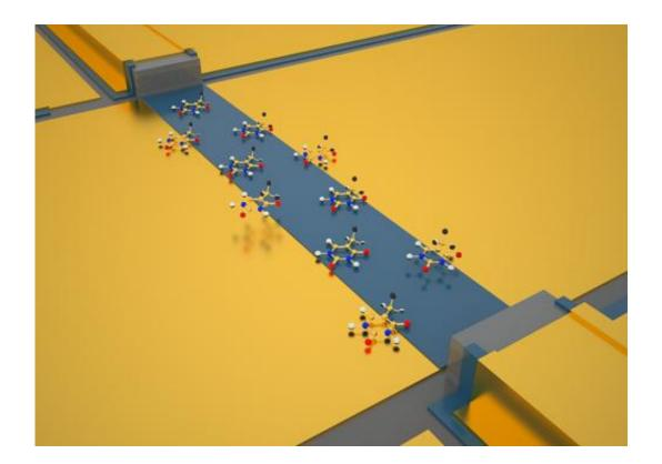
The light is emitted by the laser (top), transported on the plasmonic waveguide (blue) and hits the detector (bottom right). How much of it is absorbed depends on the chemical composition of the liquid.
