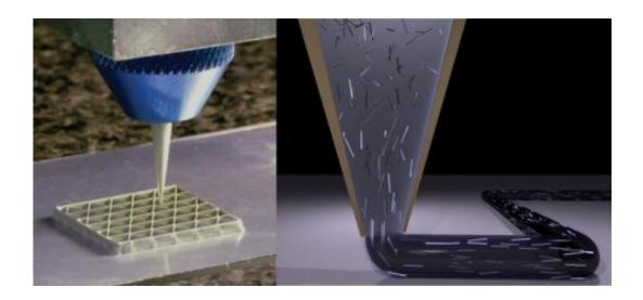
Left: Optical image of 3D printing of a triangular honeycomb composite. Right: Schematic illustration of the progressive alignment of high-aspect-ratio fillers within the nozzle during composite ink deposition. Credit: Brett G. Compton, Harvard University.
