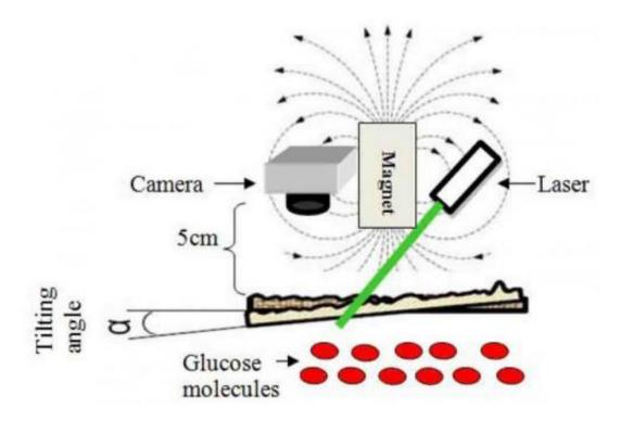
This schematic diagram shows how the new system can be used to measure a person's glucose levels non-invasively. Credit: *Biomedical Optics Express*.
