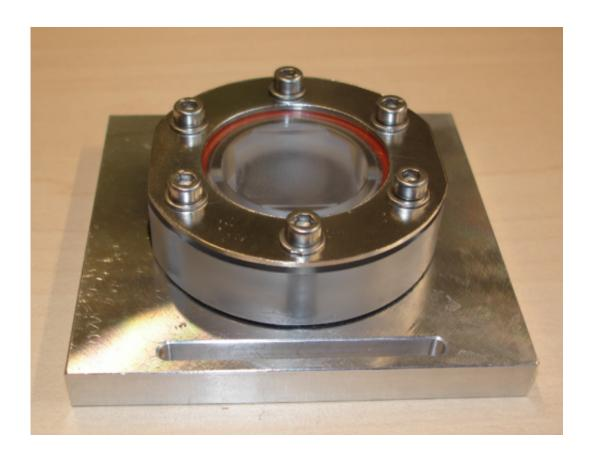
To test their pulse monitoring technique, researchers built a device that mimics blood pulsing through a person's veins under their skin. Milk was pumped through the device to mimic the blood flow, and a type of plastic called Delrin was used to mimic skin's light-scattering properties. Pitured is the blood vessel mimic ("flow cell"). Credit: Mahsa Nemati.
