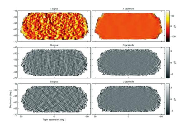
BICEP2 T, Q, U maps. The left column shows the basic signal maps with 0.25° pixelization as output by the reduction pipeline. The right column shows difference (jackknife) maps made with the first and second halves of the data set. No additional filtering other than that imposed by the instrument beam (FWHM 0.5°) has been done. Note that the structure seen in the Q and U signal maps is as expected for an E-mode dominated sky. Credit: American Physical Society
