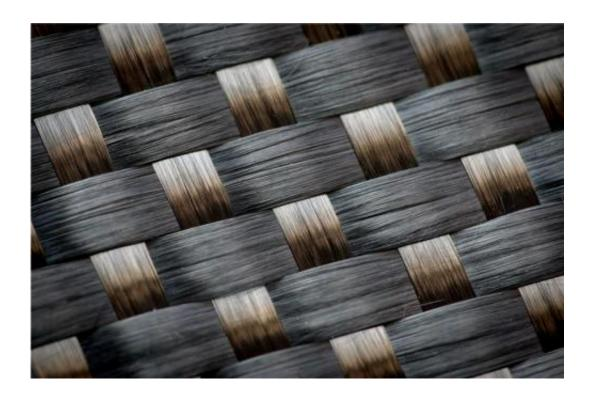
Woven carbon fibre can act as an electrode for lithium ion batteries. Credit: Peter Larsson
