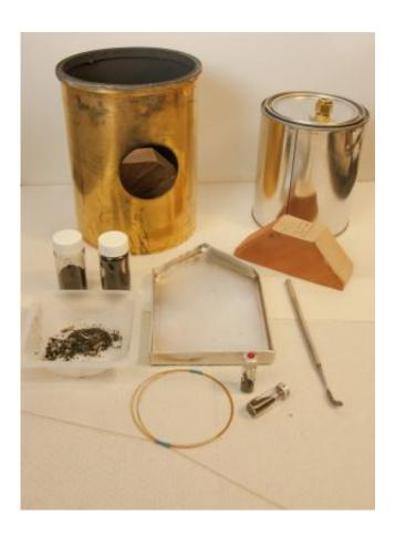
Shown here are the tools for testing arson samples using NIST's new PLOT capillary method. Clockwise from top are a test chimney with burned sample of Douglas Fir (used in test burns), paint can equipped with a septum cap, test sample of Douglas Fir, scraper, collection tray, fire debris samples, then at the bottom a PLOT capillary and two containers used with the capillary. Credit: Burrus/NIST
