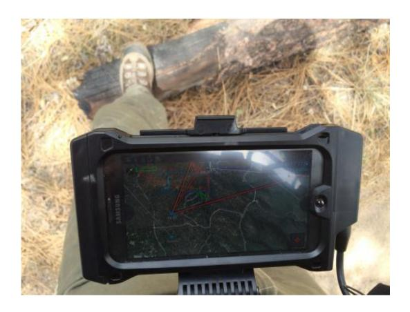
The FLASH prototype system includes a ruggedized tablet computer and MANET-capable radio that firefighters and other responders can wear, freeing
