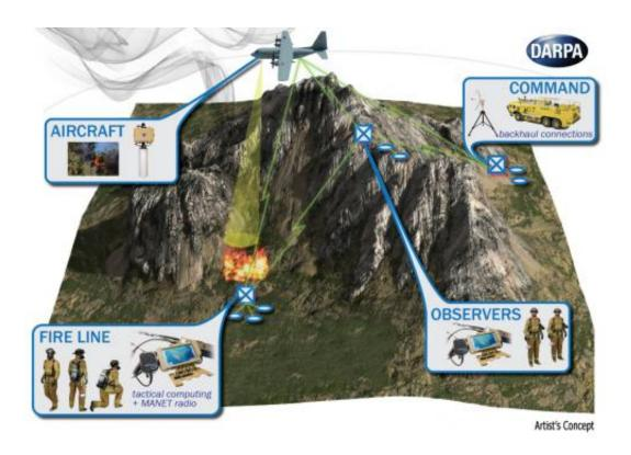
Fire Line Advanced Situational Awareness for Handhelds (FLASH) is a prototype technology system designed to improve firefighter effectiveness and safety by providing real-time situational awareness to every firefighter and firefighting aircraft in expansive fire zones. Adapted from DARPA's Persistent Close Air Support (PCAS) technology, FLASH overlays multiple streams of information from airborne sensors, firefighters and fire command posts onto a shared digital map visible via tablet computers.
