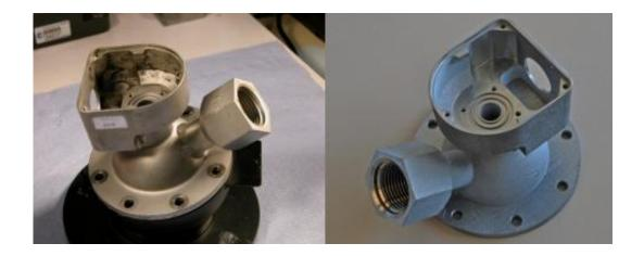
Original and 3D-printed version of the water on-off valve (Woov) flown aboard ESA's Columbus module attached to ISS. Originally made in stainless steel with a single weld and thin walls, the Additive Manufacturing demonstration version was instead manufactured in titanium with a 40% mass reduction. Credit: ESA
