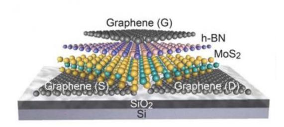
Berkeley Lab researchers fabricated the first fully 2-D field-effect transistor from layers of molybdenum disulfide, hexagonal boron nitride and graphene held together by van der Waals bonding. Credit: Ali Javey, Berkeley Lab
