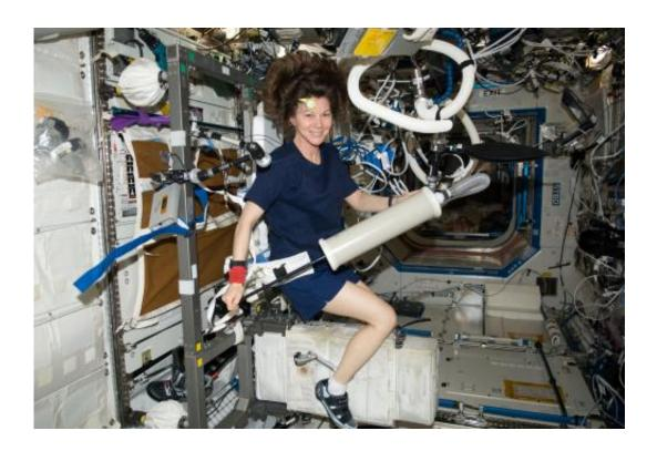
Expedition 26's Cady Coleman (NASA) calibrates a device intended to measure oxygen production while sitting on the Cycle Ergometer with Vibration Isolation System (CEVIS) in the Destiny laboratory of the International Space Station. Credit: NASA
