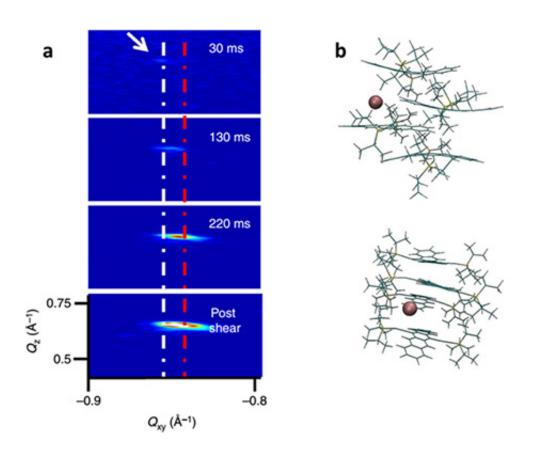
Left: Evolution of the organic semiconductors' equilibrium structure (top) to the strained structure (bottom) in the light of CHESS X-rays. Right: Cornell researchers' molecular simulations show that even a single solvent molecule (sphere) can significantly distort the molecular configuration of the surrounding organic semiconductor molecules (green). Credit: Gaurav Giri and Kristina Lenn
