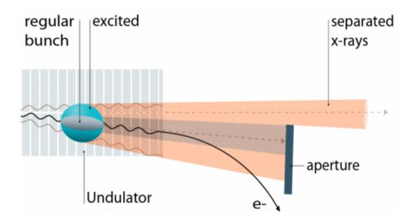
In regular operation the non-excited bunches (grey) emit undulator radiation onaxis. A detour in the electron beam (bump) makes that this regular radiation is emitted off-axis and dumped into an aperture. Only the part of the radiation from a quasi-resonantly excited bunch (blue) can enter the beamline mimicking a turn-by-turn single bunch emission. Credit: Ela Strickert/HZB
