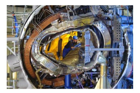
At the end of 2011 the inner life of Wendelstein 7-X was still visible. From the centre outwards: the plasma vessel, one of the twisted stellarator coils, a planar coil, the support structure (on the right) and the outer vessel together with numerous power distributors and cooling pipes. Credit: IPP, Wolfgang Filser
