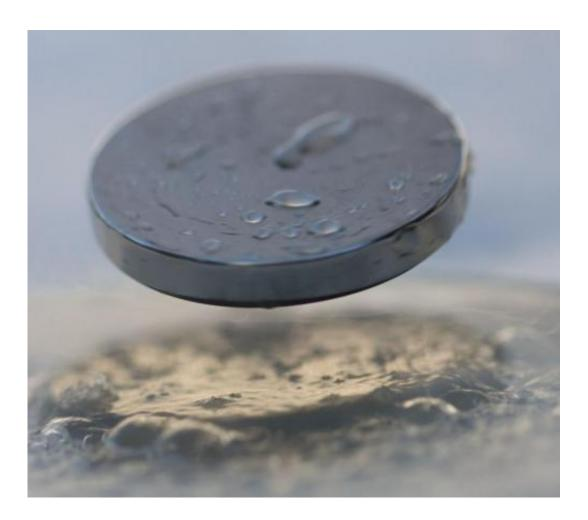
Superconducting materials expel magnetic fields, whose repulsive force can levitate a magnet, as shown here. Nevertheless, studies have shown superconductivity and magnetism can coexist in the same material. Now SLAC and Stanford researchers show that the two phases are interwoven at a very fine, microscopic level in a type of high-temperature superconductor known as an iron
