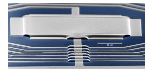
The tiny aluminum device—only 40 microns long and 100 nanometers thick—in which Caltech researchers observed the quantum noise from microwaves. Credit: Chan Lei and Keith Schwab/Caltech
