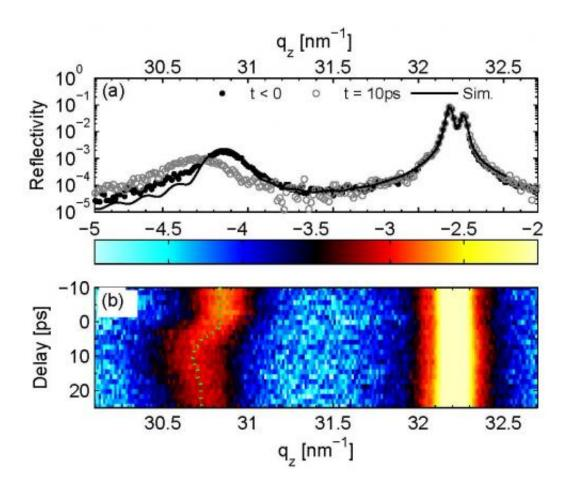
The transient  $\theta/2\theta$  scans reveal a maximum shift of the BiFeO<sub>3</sub>002 Bragg peak around 30.8 nm-1 to smaller values of the scattering vector qz within 10ps while the substrate SrTiO<sub>3</sub> peak at 32.2 nm-1 remains unchanged. (a) The black dots and gray circles correspond to slices of (b) at t
