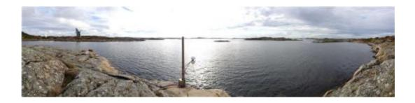
A panorama from the GNSS tide gauge at Onsala Space Observatory. When satellites pass over the sky, the GNSS tide gauge uses signals direct from the satellite and signals reflected off the sea surface to measure the sea level. Credit: Johan Löfgren
