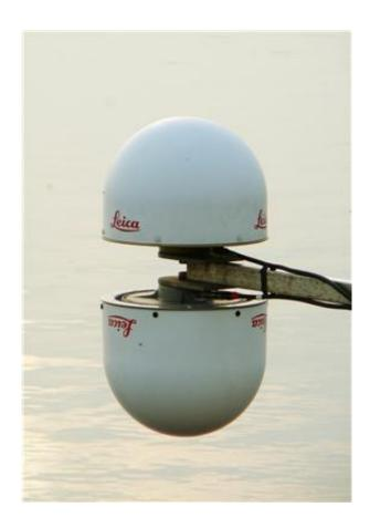
The GNSS tide gauge at Onsala Space Observatory uses signals from satellite navigation systems like GPS to measure the sea level. Credit: Johan Löfgren
