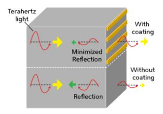
Thin strips of chromium form an efficient antireflection coating for terahertz light and can be applied to a broad range of surfaces. Credit: A\*STAR Institute of Materials Research and Engineering
