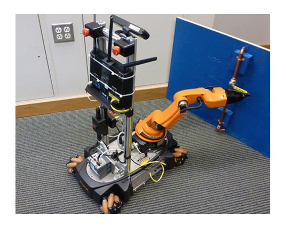
This robot has a mounted camera and router to transmit the robot's view of the scene, and built-in haptics technology allows the operator to receive force feedback from the robot. Credit: U of Washington
