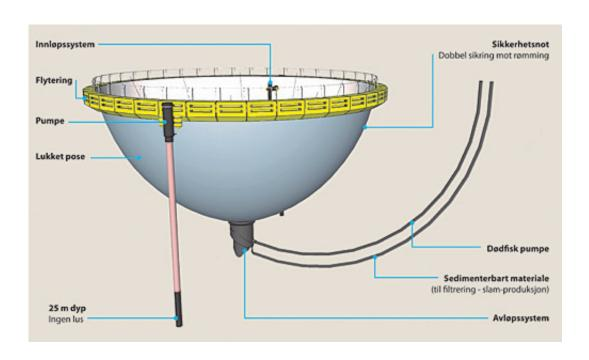
Conceptual draft of a closed cage. Credit: Akva Design AS
