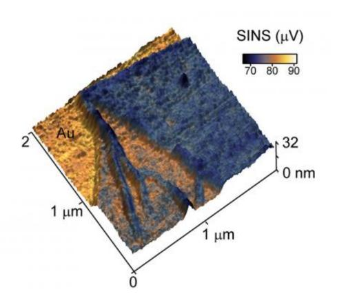
This peptoid nanosheet, produced by Gloria Olivier and Ron Zuckerman at Berkeley Lab, is less than 8 nanometers thick at points. SINS makes it possible to acquire spectroscopic images of these ultra-thin nanosheets for the first time. Credit: Berkeley Lab
