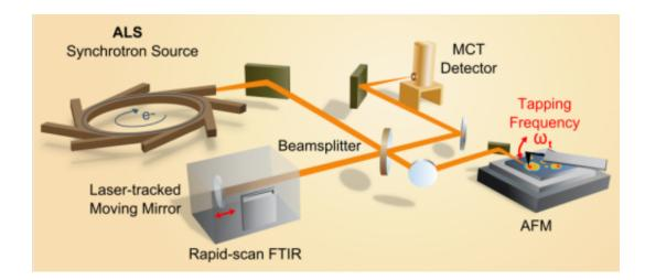
Experimental setup for SINS that includes the synchrotron light source, an atomic force microscope, a rapid-scan Fourier transform infrared spectrometer, a beamsplitter, mirrors and a detector. Credit: Berkeley Lab
