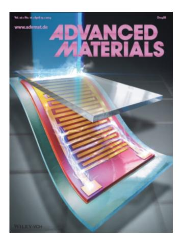
This picture shows a flexible PZT thin film nanogenerator using inorganic-based laser lift-off process. Credit: KAIST
