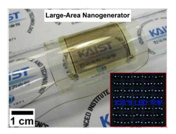
This is a photograph of large-area PZT thin film nanogenerator  $(3.5 \text{ cm} \times 3.5 \text{ cm})$  on a curved glass tube and 105 commercial LEDs operated by self-powered flexible piezoelectric energy harvester. Credit: KAIST
