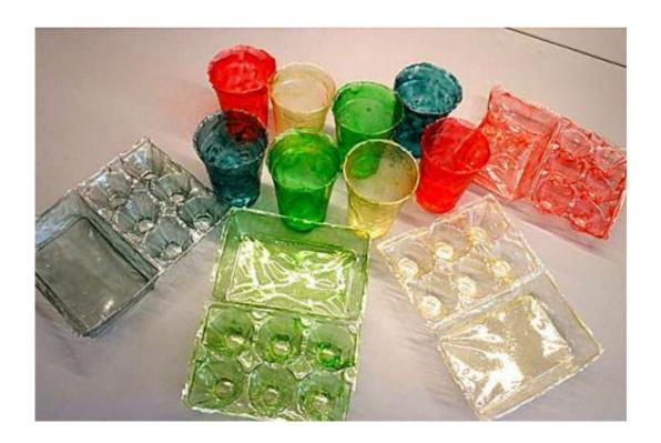
Turning shrimp shells into plastic: Harvard's Wyss Institute comes up with fully degradable bioplastic. Credit: Wyss Institute
