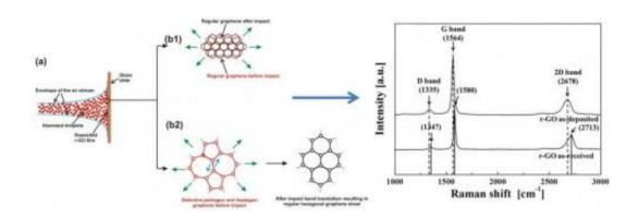
Using a supersonic spray, graphene flakes with deformed pentagonal and heptagonal structures stretch on impact and spring into a perfect hexagonal graphene lattice. This opens the way to scale up from the microscopic to large scale applications. Credit: Photo credit: Suman Sinha-Ray
