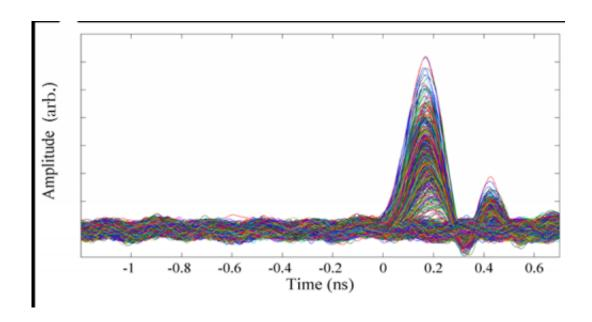
Output signals from the detection system (after a low-noise output amplifier), showing both avalanches and the background noise floor. The noise floor allows the use of a minimum threshold below 2 mV in a 5GHz bandwidth. As can be seen, nearly all avalanches can be discriminated from the noise floor.
