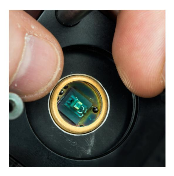
SPADs are typically small. Here a unit used in testing is seen at the center of the round aperture.
