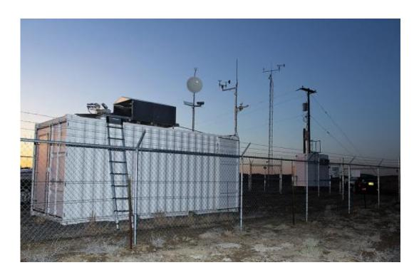
Measurement devices in place near the Four Corners coal-fired power plant, allowing Los Alamos National Laboratory researchers to analyze emissions.
