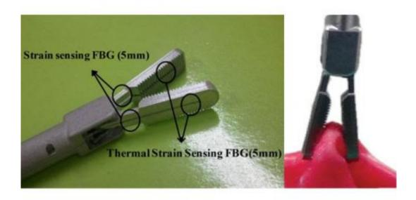
A closer look at the grip force sensing forceps with their embedded FBGs (L) and in use, gripping a test material (R)
