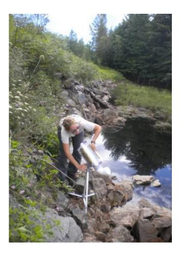
Laci Coleman: Laci Coleman places acoustic monitoring equipment to detect the presence of bats near a wetland on Fort Drum, N.Y.
