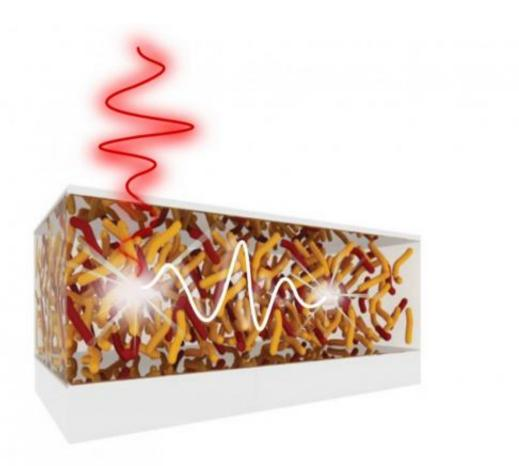
This is the device trapping photons between two mirrors in which two different organic molecules reside. Credit: University of Southampton
