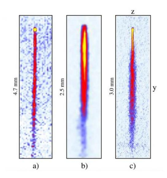
The new atom laser technique can be used to create different types of lasers. These figures show the atom density distributions of (a) a well-collimated atom laser beam, (b) an ultra-high flux atom laser, and (c) an atom beam combining an
