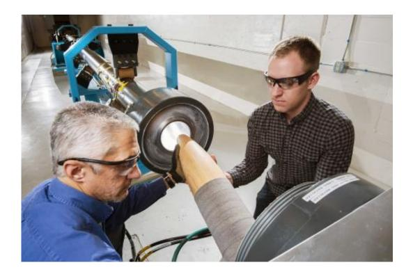
The Mechanical Shock Facility is Sandia's oldest environmental test facility. The construction team added a six-inch bore gas gun, seen here with researchers Adam Slavin, left, and Patrick Barnes. Credit: Randy Montoya
