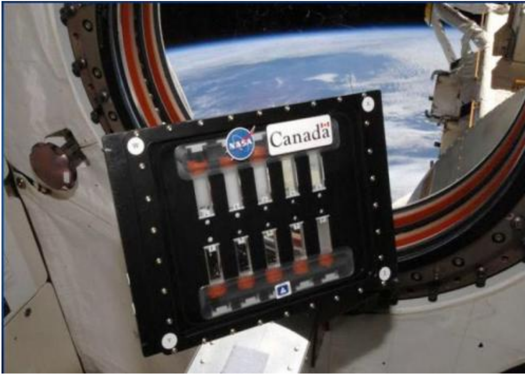
This is a BCAT-5 Slow Growth Sample Module in a window of the International Space Station. Credit: NASA/CSA
