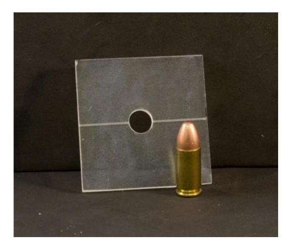
Image of a damage hole in a thin epoxy sheet that is 9 mm in diameter, next to a 9 mm bullet. The restorative system was able to recover damage sizes up to 9 mm in diameter, making it possible to restore synthetic materials that undergo catastrophic damage events such as ballistic impact by autonomously replacing lost mass. Credit: Brett Krull, University of Illinois
