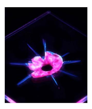
Illinois researchers have developed materials that not only heal, but regenerate. The restorative material is delivered through two, isolated fluid streams (dyed red and blue). The liquid immediately gels and later hardens, resulting in recovery of the entire damaged region. This image is halfway through the restoration process. Credit: Ryan Gergely
