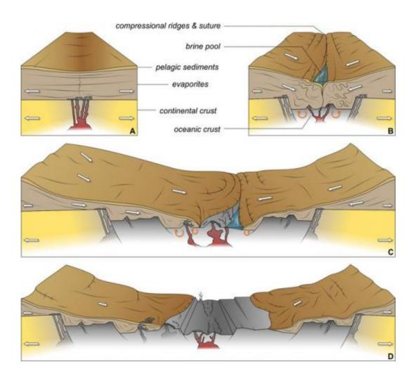
Schematic representation of the break-up of the Red Sea. In some places, salt glaciers pushed across the fault line and cover parts of the continuous rift zone, even today. Credit: N. Augustin, GEOMAR
