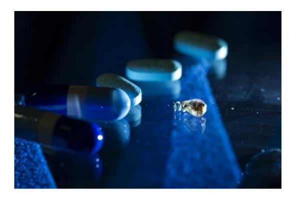
A batteryless electrostimulator next to medicinal pills for size comparison. The new powering method allows the device to be wirelessly powered deep inside the body, in locations such as the heart or brain. Credit: Austin Yee.
