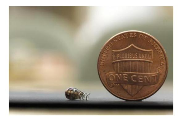
A batteryless electrostimulator next to a US penny for size comparison. The new powering method allows the device to be wirelessly powered deep inside the body, in locations such as the heart or brain. Credit: Austin Yee.
