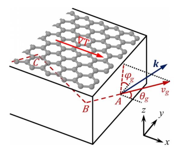
Schematic to model phonon scattering by boundary in a multilayer graphene ribbon where the group velocity and wave vector are not collinear because of the highly anisotropic structure. Credit: Li Shi, The University of Texas at Austin
