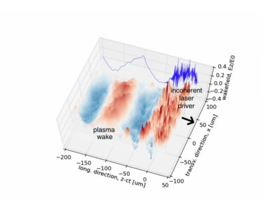
This is a 3D map of the longitudinal wakefield generated by the incoherent combination of 208 low-energy laser beamlets. In the region behind the driver, the wakefield is regular. Credit: Carlo Benedetti, Berkeley Lab
