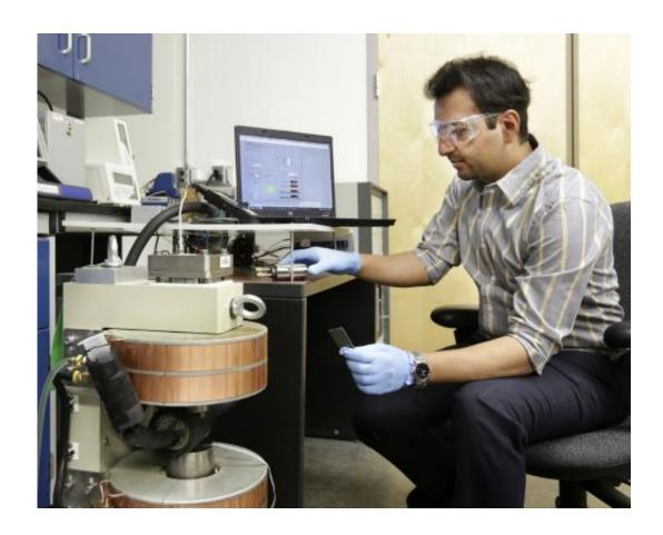
ORNL's Ayyoud Momen works on the team's "breadboard" prototype refrigerator-freezer: a flexible platform used to evaluate material compatibility and to analyze components including the magnet, generators, motor, pump, heat exchangers, plumbing and leakless rotating valve.
