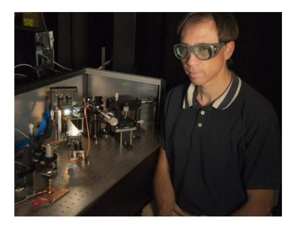
NIST engineer Tasshi Dennis with NIST's solar simulator based on a white light laser. The instrument simulates sunlight to help measure the properties of solar cell materials. The instrument's beam is illuminating a gallium arsenide solar cell (yellow diamond) in the lower left corner of the photo. Credit: J. Burrus/NIST
