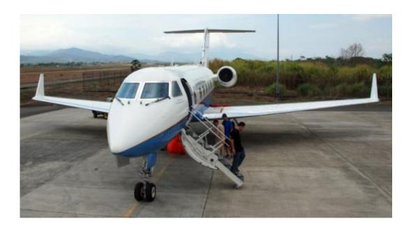
NASA's C-20A aircraft crew preparing for flight from Tocumen International Airport in Panama City, Panama. The aircraft was deployed to Central and South America for a research study using JPL's UAVSAR airborne radar, located in an underbelly pod (note red cover). Credit: NASA/Armstrong Flight Research Center
