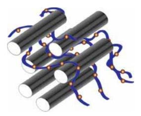
Single-walled carbon nanotubes, represented by the gray cylinders, can be combined with a catalyst (purple ribbons) that is capable of breaking down Sarin and related toxins into less dangerous components. The idea might one day be used to create clothing for increased protection against nerve agents.
