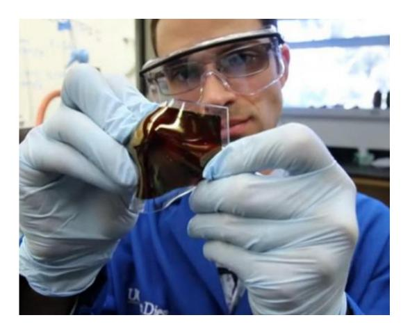
Nanoengineering professor Darren Lipomi is developing new "molecularly stretchable" electronic materials for applications in energy, biomedical devices, wearable sensors and consumer electronics. Credit: Darren Lipomi, UC San Diego Jacobs School of Engineering
