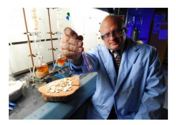
Professor Arthur Ragauskas prepares samples containing cellulose, lignin and hemicellulose for analysis using advanced nuclear magnetic resonance techniques. Credit: Gary Meek
